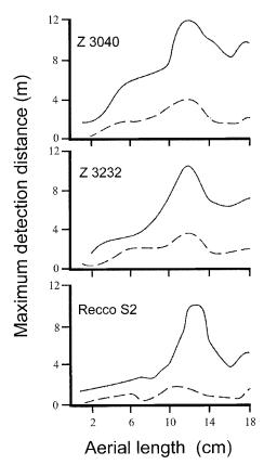
Figure 1: Maximum detection range of the diodes Z 3040, Z 3232, and Recco S2 with different aerial lengths in parallel (solid line) and perpendicular (broken line) orientation to the radar beam. The aerial was always attached to the cathode end of the diode.
