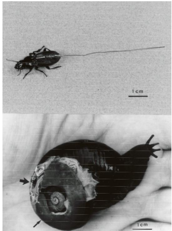
Figure 2: Two invertebrates fitted with a Schottky-type diode and appropriate aerial for harmonic radar studies. Top: a female carabid beetle, *Plocamosthetus planiusculus*. Bottom: the snail *Paryphanta busbyi wattii*. Note the different aerial shapes. The thick arrow points to the diode, the narrow one to the aerial.
