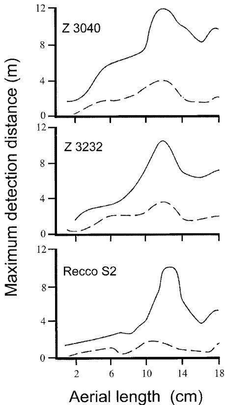
Figure 1: Maximum detection range of the diodes Z 3040, Z 3232, and Recco S2 with different aerial lengths in parallel (solid line) and perpendicular (broken line) orientation to the radar beam. The aerial was always attached to the cathode end of the diode.
